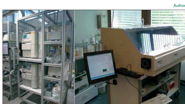
Fig. 2a and b: Modular and mobile equipment rack at Merck Serono, Geneva (left); Mobile bioreactor at the Lab Innovation Center, Fraunhofer Institute for Interfacial Engineering and Biotechnology IGB, Stuttgart (right)
